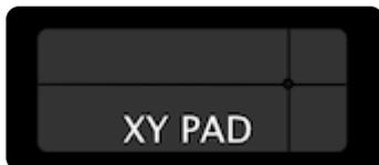
Like Envelopes, XY Pads are multi-value controls. That means they represent more than one MIDI parameter — in this case, two. By default, only one axis (X or Y) is assigned to the knob at a time. You can configure which one is active by default and switch between them as needed while using the preset. This allows you to fine-tune each parameter individually using the knob, while still having full dual-axis control through touch.
