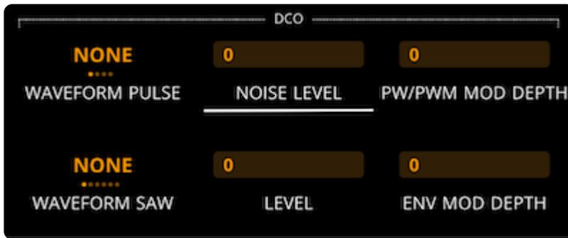
You can change a control’s value by turning the corresponding knob, or by swiping left or right on the control directly on the touchscreen.
