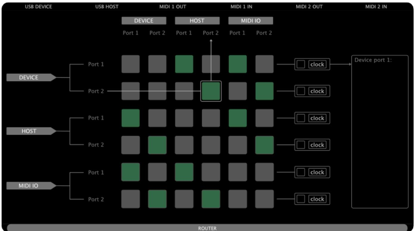
As shown, each MIDI interface forwards both of its ports to the corresponding ports on the other two interfaces.
