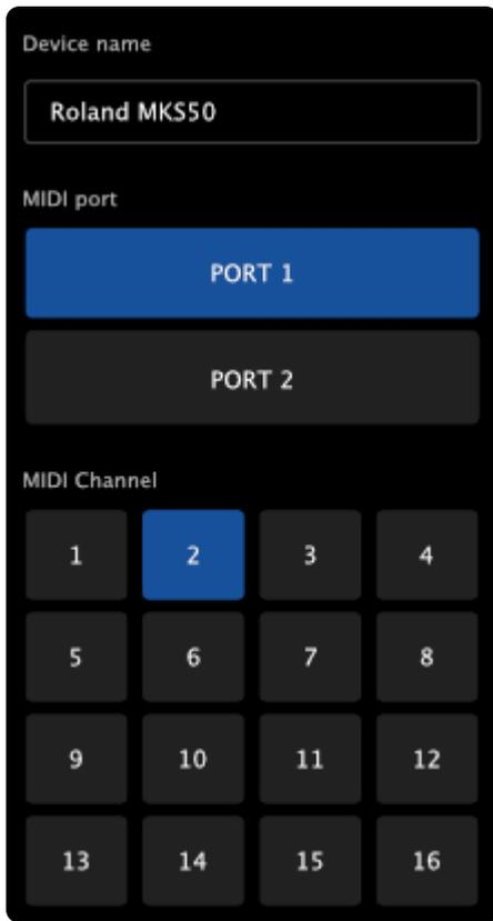
To select another device, simply tap its entry. Note that you cannot select unused channels. The form is easy to use - just tap the MIDI Port and Channel you want to assign. If the selected combination is already used by another device, the controller will swap the devices to accommodate the change.
