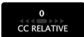
The visual appearance of a Relative Control reflects this behavior. It does not display the actual value of the parameter. Instead, it shows a momentary indication of how much the value changes when the knob is turned.
